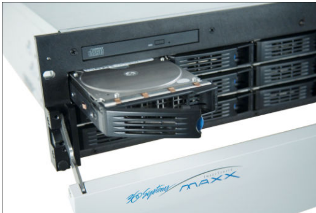
Figure 45 - Front Panel Opened – Disk Unlatched
